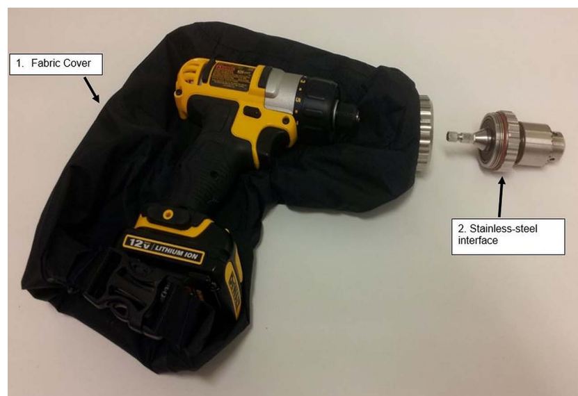
Figure 1 The drill cover system is composed of a hardware drill plus two detachable parts. The fabric cover (1) is constructed of a double-layered medical fabric typically used for surgical drapes and gowns. The stainless-steel interface (2) comprises a shaft, three-tooth adjustable chuck and encased bearings that enable the operator to use various sizes of surgical drill bits.
